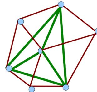
The cell is modeled as a collection of points (beads) connected by springs, which approximate both kinds of tensegrity components but with simple computations of changes. The parameters of the springs are the undeformed length and the elasticity; a strut has low elasticity, a cable high elasticity.
